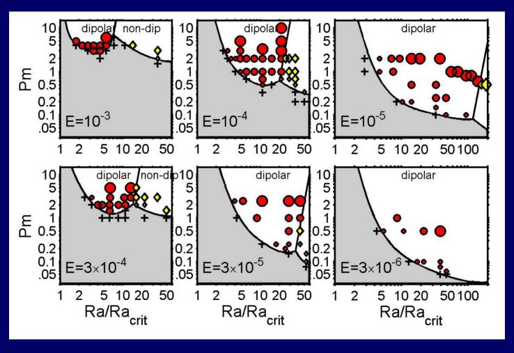
As the Ekman number is lowered, dipolar dynamos occupy a broader region and are found at lower magnetic Prandtl #
