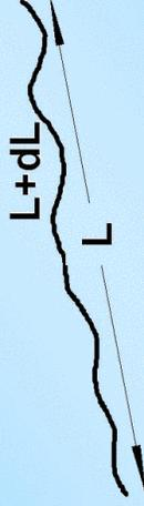
Elastic energy difference between a crack of length L and length L+dL is
