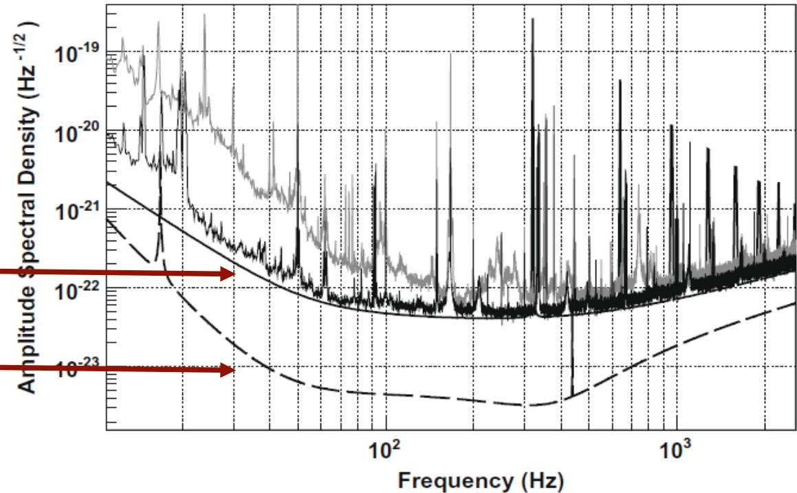
Shot noise (random photon emissions), photons shake the mirrors, earthquakes,...
