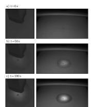
Jet Speed at bed:  $w_j = 4.0 \text{ cm/s}$ , Setting Speed:  $W_s = 0.66 \text{ cm/s}$ Shields Number: Sh = 2.4, Rouse Number: Rs = 0.41
