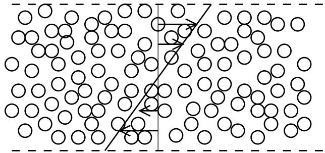
Balance between shear production  $\dot{\phi}$  and inelastic dissipation.
