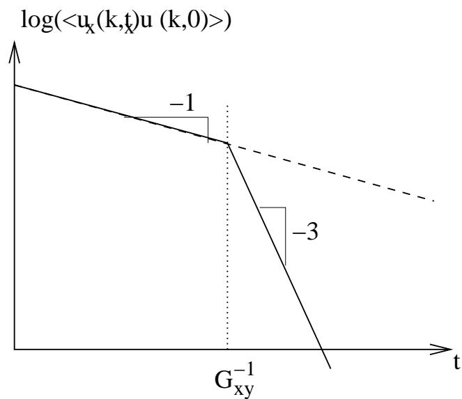
$$u_x(t) = u_x(0) \exp \left[ -Dt \left( k^2 - G_{xy} t k_x k_y + \frac{1}{3} G_{xy}^2 t^2 k_x^2 \right) \right]$$
