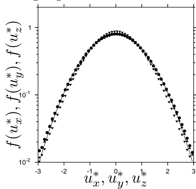
Rough particles,  $\phi = 0.56$ ,  $e_n = 0.98$  ( $\circ$ ),  $e_n = 0.8$  ( $\triangle$ ),  $e_n = 0.6$  (Box).
