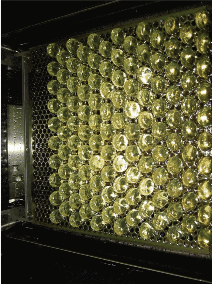
Stereolithography for 1.25:1:0.8 ellipsoids
