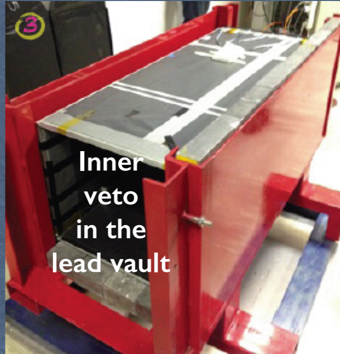
Inner veto plastic scintillators paddle + WLS + SiPM
