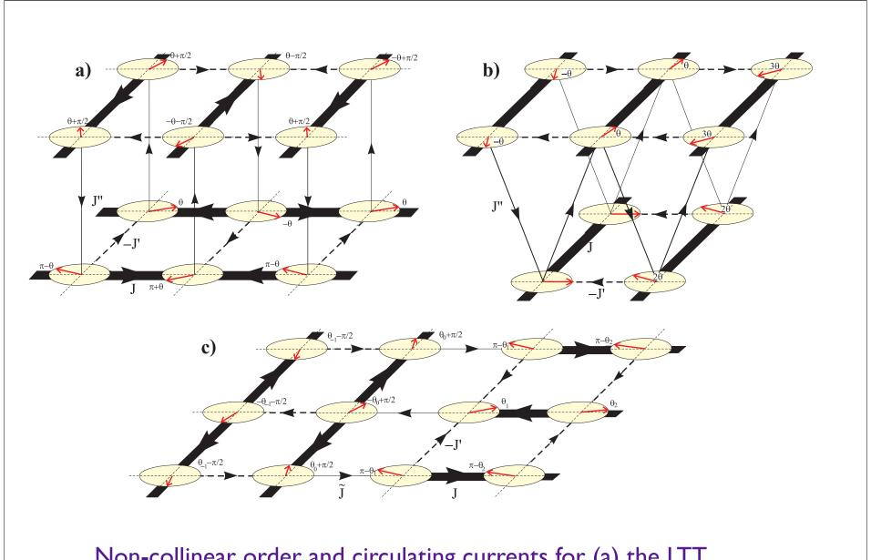
Non-collinear order and circulating currents for (a) the LTT structure (LBCO), (b) the orthorhombic (chain) structure of YBCO, and (c) an in-plane domain wall ("twin boundary").
