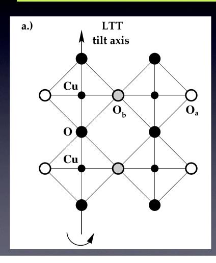
The tilt in the oxygen octahedra induces a different t and J along x and y:
