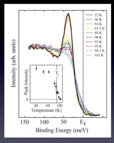
(pi,0) vs.T Fedorov 1999 Bi2212 Tc=91K Existence of a pseudo-gap but no superconductivity and no quasiparticles
