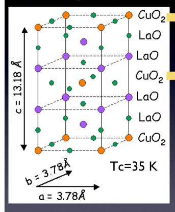
Layered structure with CuO<sub>2</sub> planes
