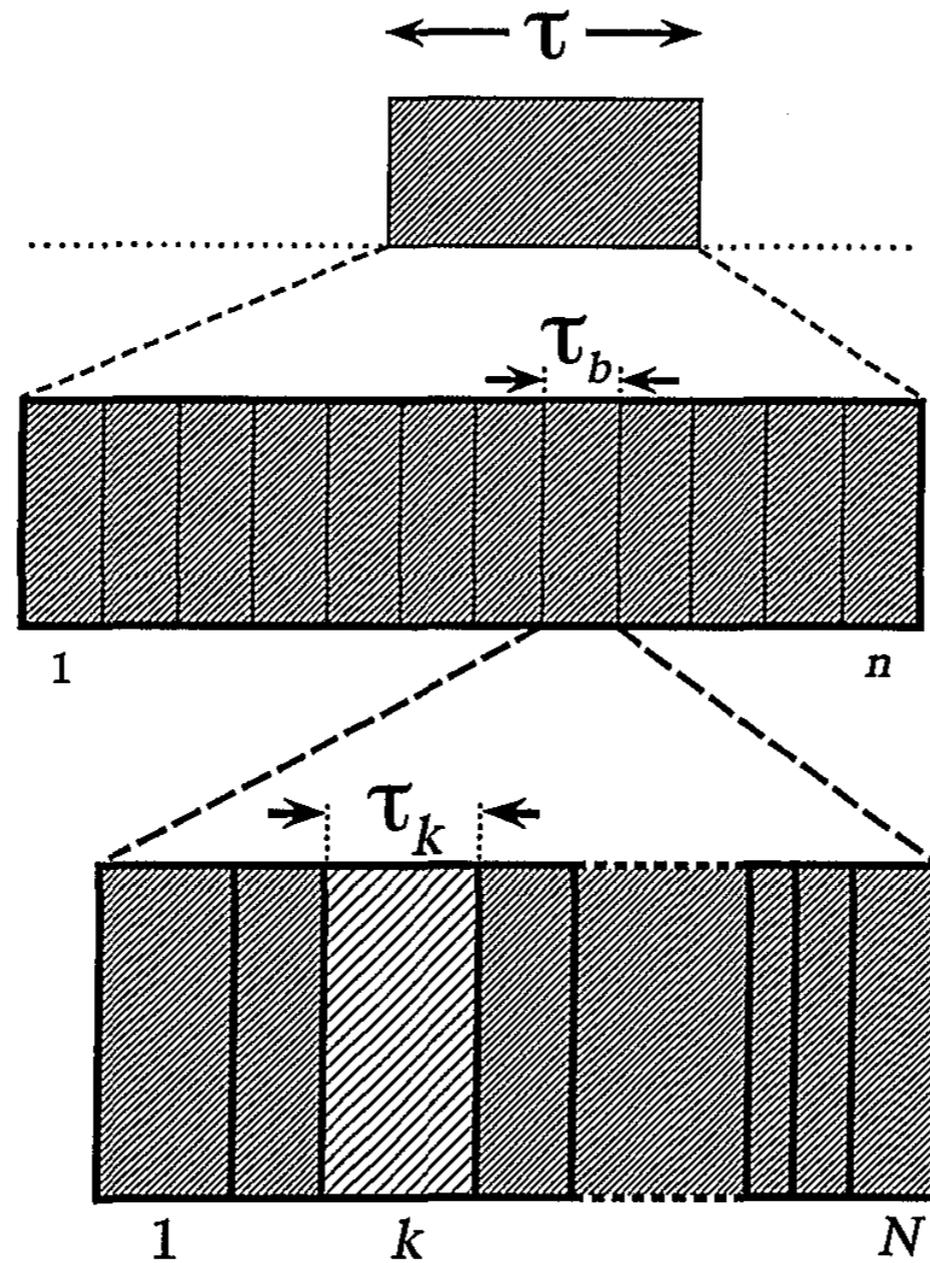
A square pulse may be completely characterized by the four parameters  $\tau_k$ ,  $\nu_k^{\text{rf}}$ ,  $B_k$ , and  $\varphi_k$  or, alternatively, by the four parameters  $\alpha_k$ ,  $\nu_k^{\text{rf}}$ ,  $\nu_k^R$ , and  $\varphi_k$ . If the flip angles, frequencies, amplitudes, and phases of all  $N$
