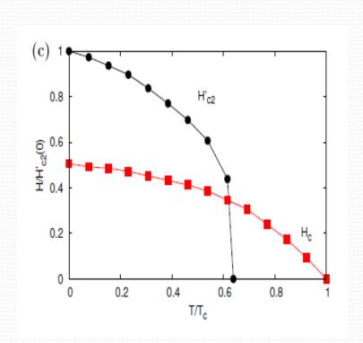
The sharp drop indicate the suppression of vortex state in small sample.
