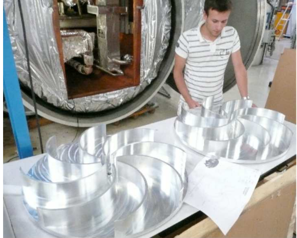
Aluminium turbines (machined from one big aluminium sheet)
