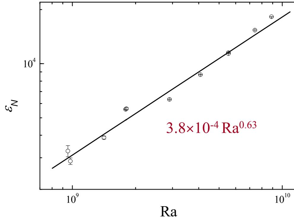
(vi)  $\epsilon_m \sim Ra^{+\beta}$  with  $\beta = 0.63 \pm 0.05$  inside the thermal boundary layer.
