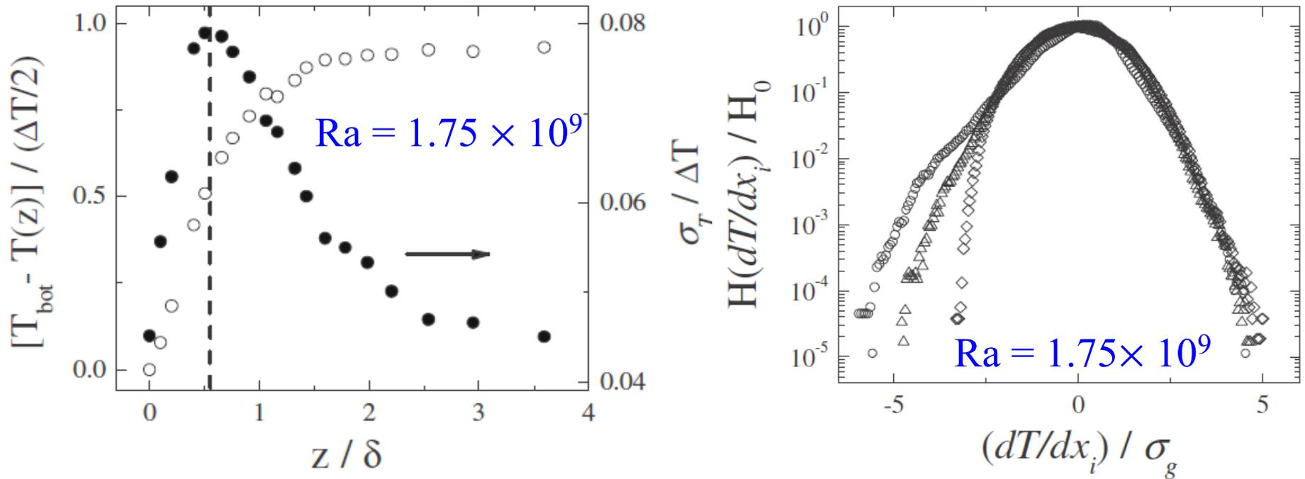
Temperature fluctuations near the lower conducting plate are governed by the thermal boundary layer thickness,  $\delta$ , which decreases with increasing  $Ra$ . Measurements were made in the peak region ( $0.5 \leq z/\delta \leq 0.9$ ).
