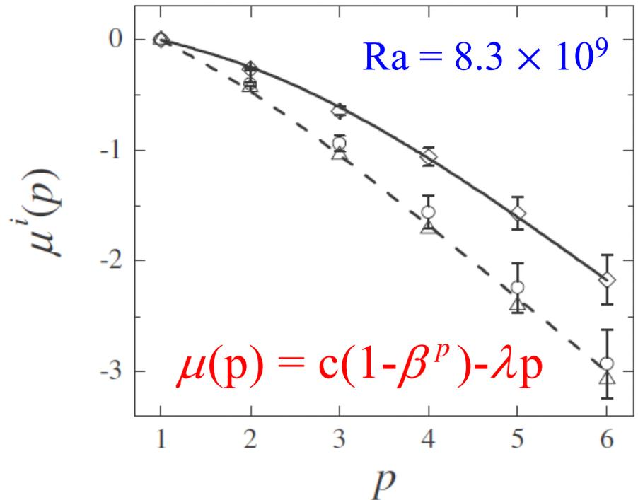
x and y components:  $c = 1$  (sheet-like),  $\beta = 1/3$  and  $\lambda = 2/3$  (passive)
