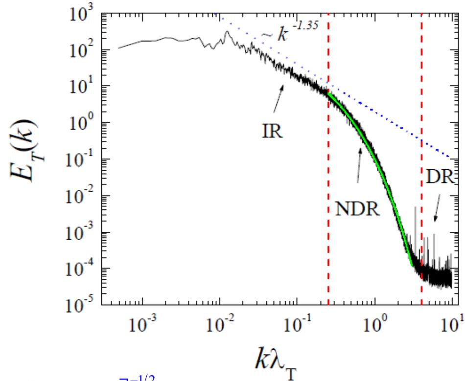
Taylor's micro-scale:  $\lambda_T = \left[ -\frac{1}{2} \frac{\partial^2 C_T(0,0)}{\partial r^2} \right]^{-1/2} = 8.53 \text{ mm}$
