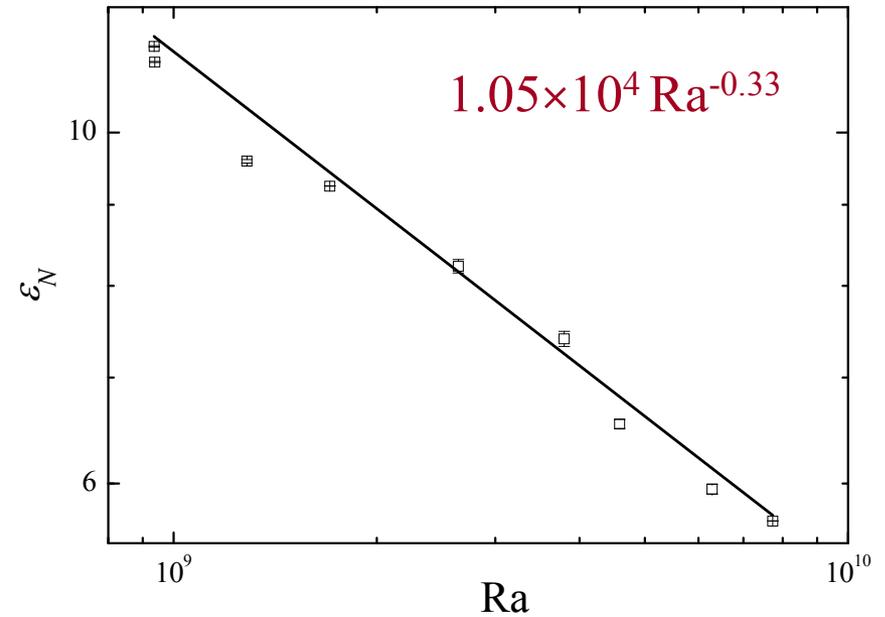
(v)  $\epsilon_f \sim Ra^{-\alpha}$  with  $\alpha = 0.33 \pm 0.03$  both at the cell center and near the sidewall.
