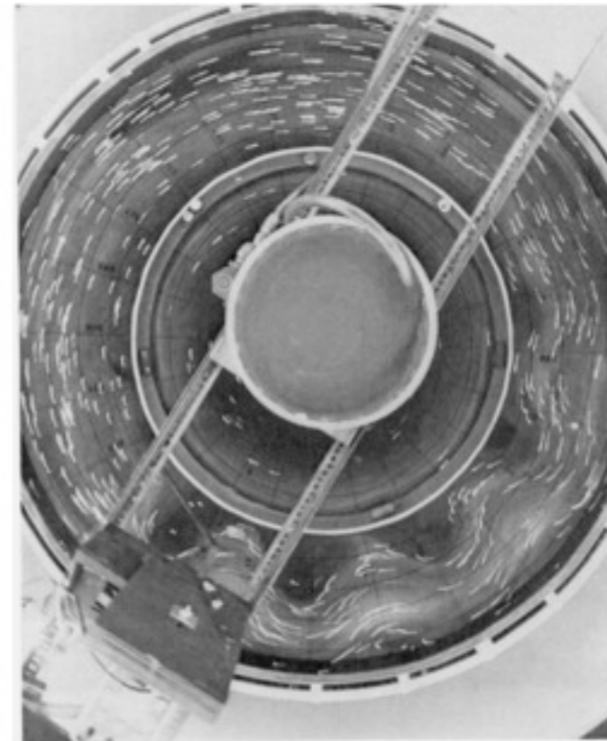
Figure 14. Stationary Rossby waves generated by an obstacle in a rotating annulus of liquid with a free surface.
