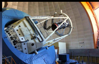
The 520 megapixel Dark Energy Camera (DECam)
