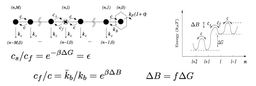
Presence of error leads to 'renormalization' of  $K \Rightarrow K^* \simeq K \bar{k}_b/k_b$
