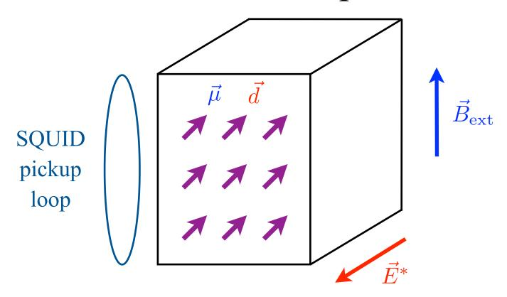
high nuclear spin alignment achieved in several systems, persists for  $T_1 \sim$  hours applied E field causes precession of nucleus
