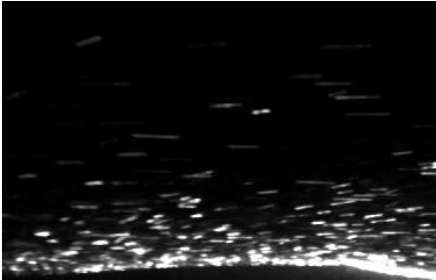
2D LASER slice of 3D sand flow inside a large wind Tunnel
