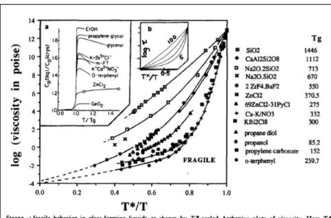
. Strong → fragile behavior in glass-forming liquids as shown by T\*-scaled Arrhenius plots of viscosity. Here T\* rature at which the shear viscosity reaches 10<sup>12</sup> Pas. Inset (a) shows how this pattern is reproduced by norm—Tammann-Fulcher equation, eq. (1), by variation of the parameter D. Inset (b) shows the corresponding configuration ponents of the heat capacity introduced at T<sub>a</sub> by ratioing the liquid (and glass) data to the crystal values at each temperation.
