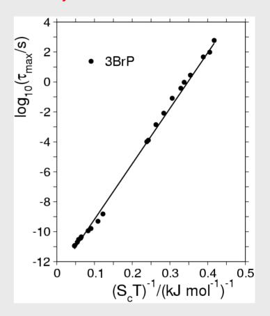
Richert and Angell (1998)  $\Rightarrow$  AG works well over a large T-and  $\tau$ -range (NB: No fit parameter!)
