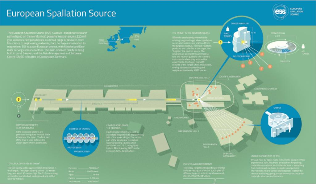
5MW long-pulsed spallation neutron source Rotating W spallation target ~3 msec pulses, 2 GeV proton linac, 14 Hz rep rate
