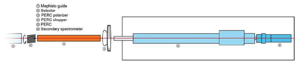
Beam (under construction) is devoted to the PERC neutron beta decay spectrometer facility
