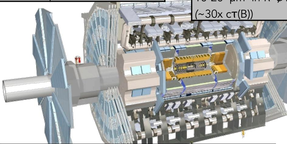
Central calorimeters (to  $|\eta| \sim 2.5$ )
