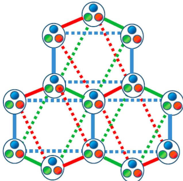
$$\mathcal{H} = K_1 \sum_{\langle ij \rangle_\gamma} S_i^\gamma S_j^\gamma + K_2 \sum_{\langle\langle ij \rangle\rangle_\lambda} S_i^\lambda S_j^\lambda$$
