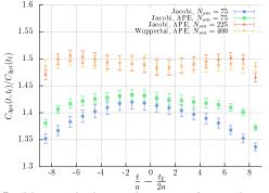
Example of a ratio of 3ptover 2pt-functions for  $g_A$ : "good" smearing vs. "not so good" smearing (not renormalized).
