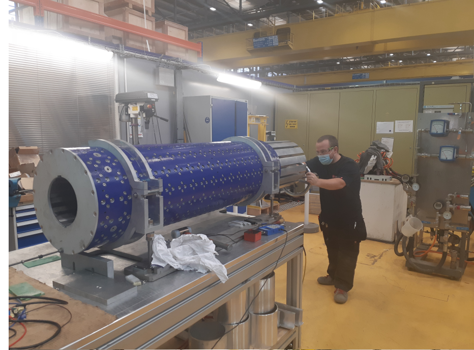
FASER permanent dipole magnets. Constructed at CERN.
