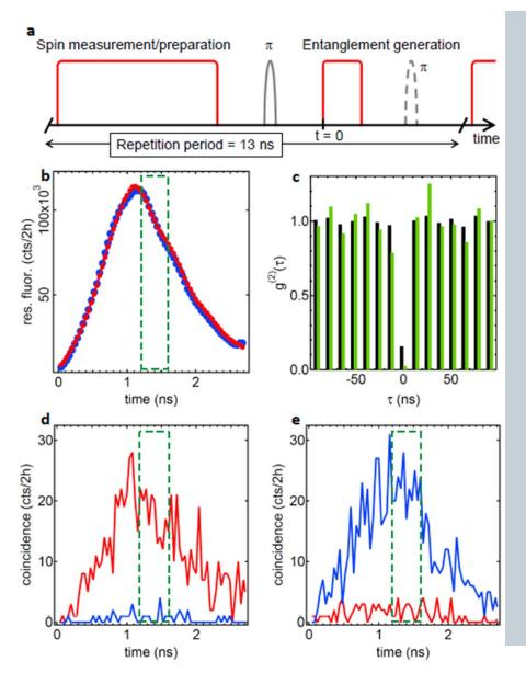
An additional  $\pi$ -pulse (dashed curve) is applied to realize a heralded measurement in the spin-up state.
