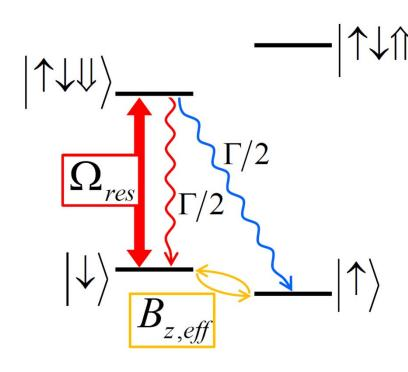
⇒ Spin-photon entanglement: potentially near-determinsitic entanglement generation at ~1 GHz rate
