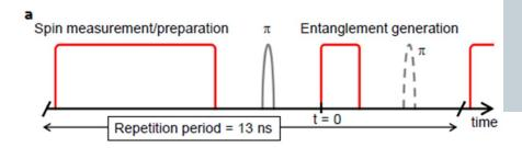
An additional  $\pi$ -pulse (dashed curve) is applied to realize a heralded measurement in the spin-up state.
