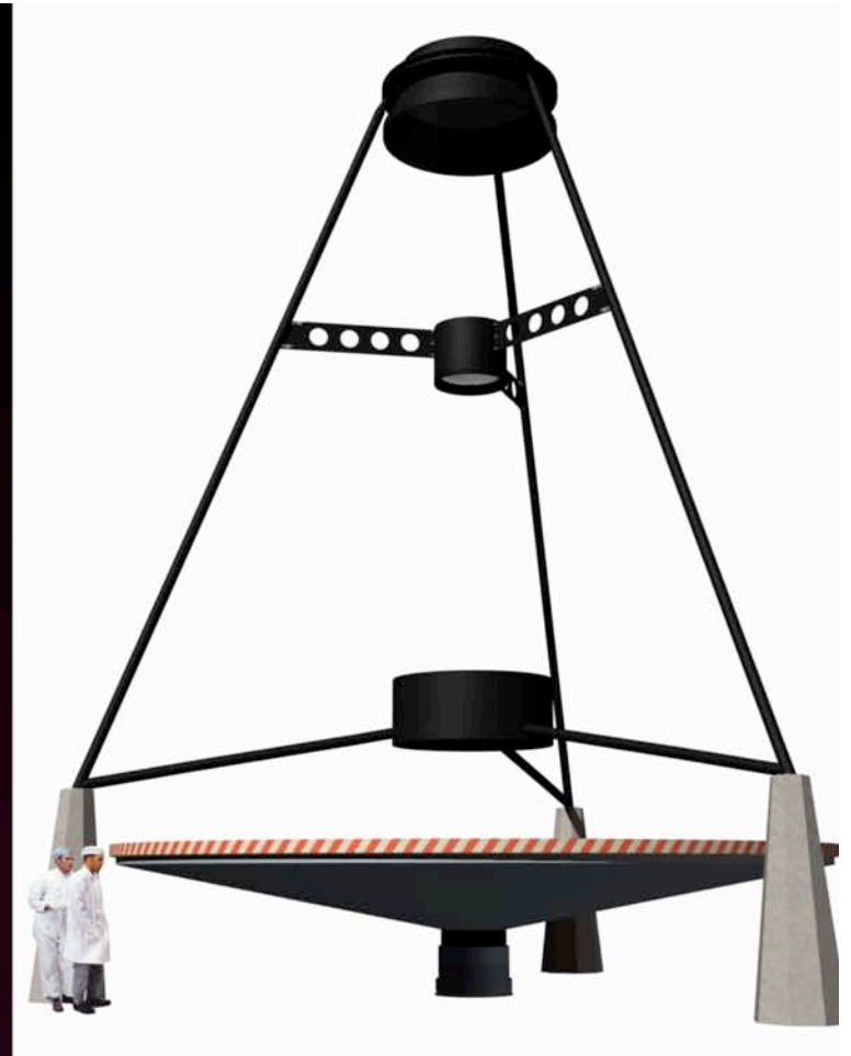
8m Spinning Mercury Mirror
