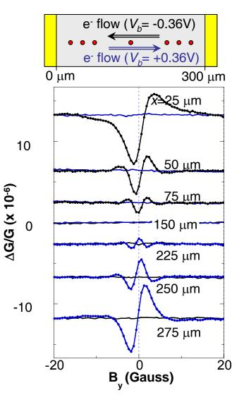
• Conductance is higher for the minority channel, consistent with the sign of the spin accumulation.
