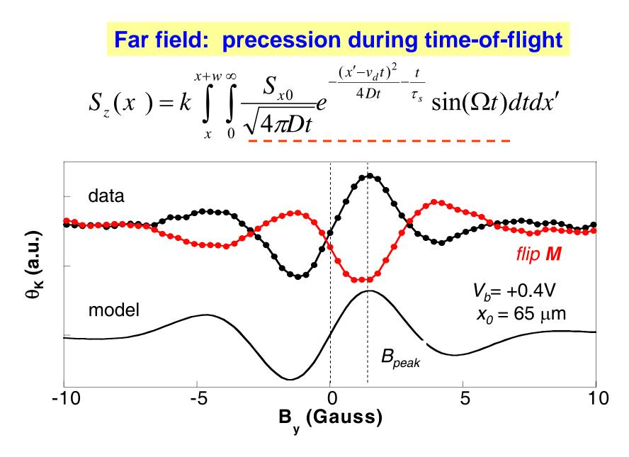
At  $x_0 = 65 \ \mu\text{m}$ ,  $B_{\text{peak}} = 1.35 \ \text{Gauss}$ ,  $T = \pi/2\Omega_L \sim 300 \ \text{ns}$ , or  $v_d \sim 2.8 \times 10^4 \ \text{cm/s}$
