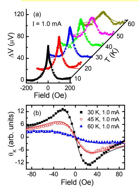
Electrical detection; curves are fits with the drift-diffusion model
