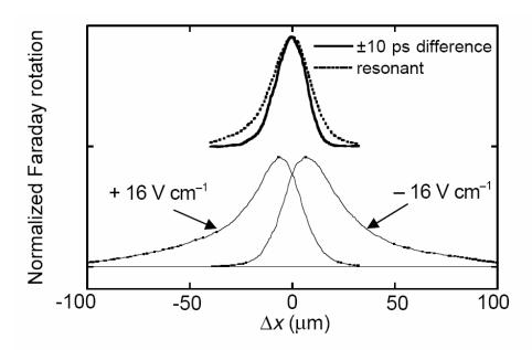
Doping:  $1-3 \times 10^{16} \text{ cm}^{-3}$ Spin drift lengths > 100 microns Diffusion constant ~ 10 cm<sup>2</sup>/s Spin lifetime: 100 nsec
