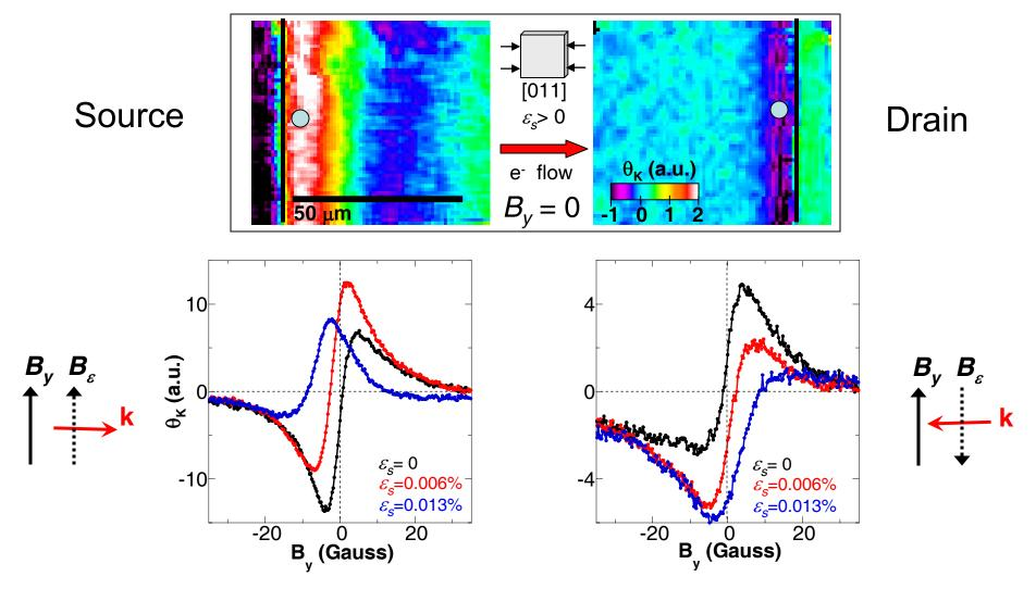
• At opposite ends of the channel, the Hanle curves shift in **opposite** directions with increasing strain. *The (diffusive) spin current at the drain is flowing against the charge current*.
