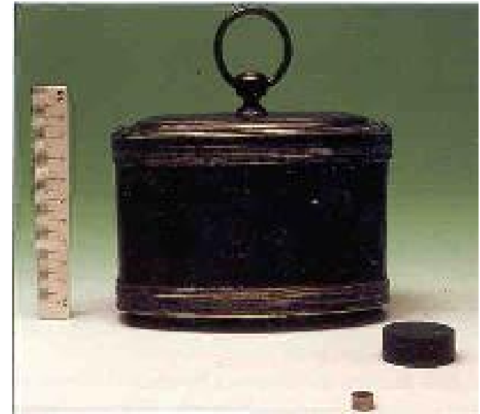
A lodestone magnet from the 1750's and typical ferrite and rare earth used in modern appliances. Each of these contain about 1J of magnetic energy.
