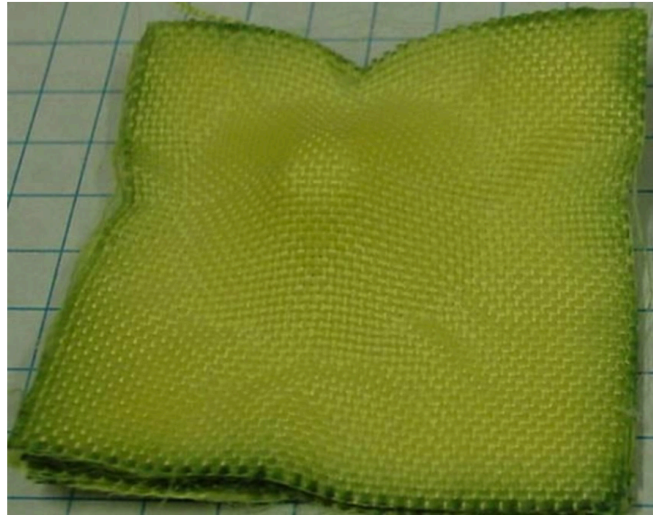
Kevlar soaked with STFluids University of Delaware (Professor Wagner) in collaboration With US Army.
